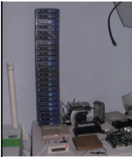
Tall Stack of Linksys Access Points to handle the 200 Conferees Wi-Fi equipped personal computers
